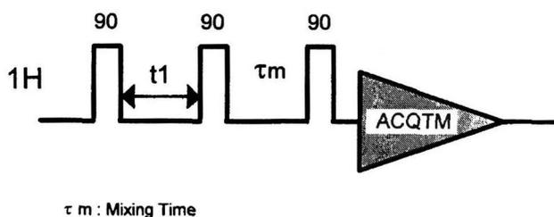
Fig. 1. Pulse sequence for PS-NOESY experiment.
