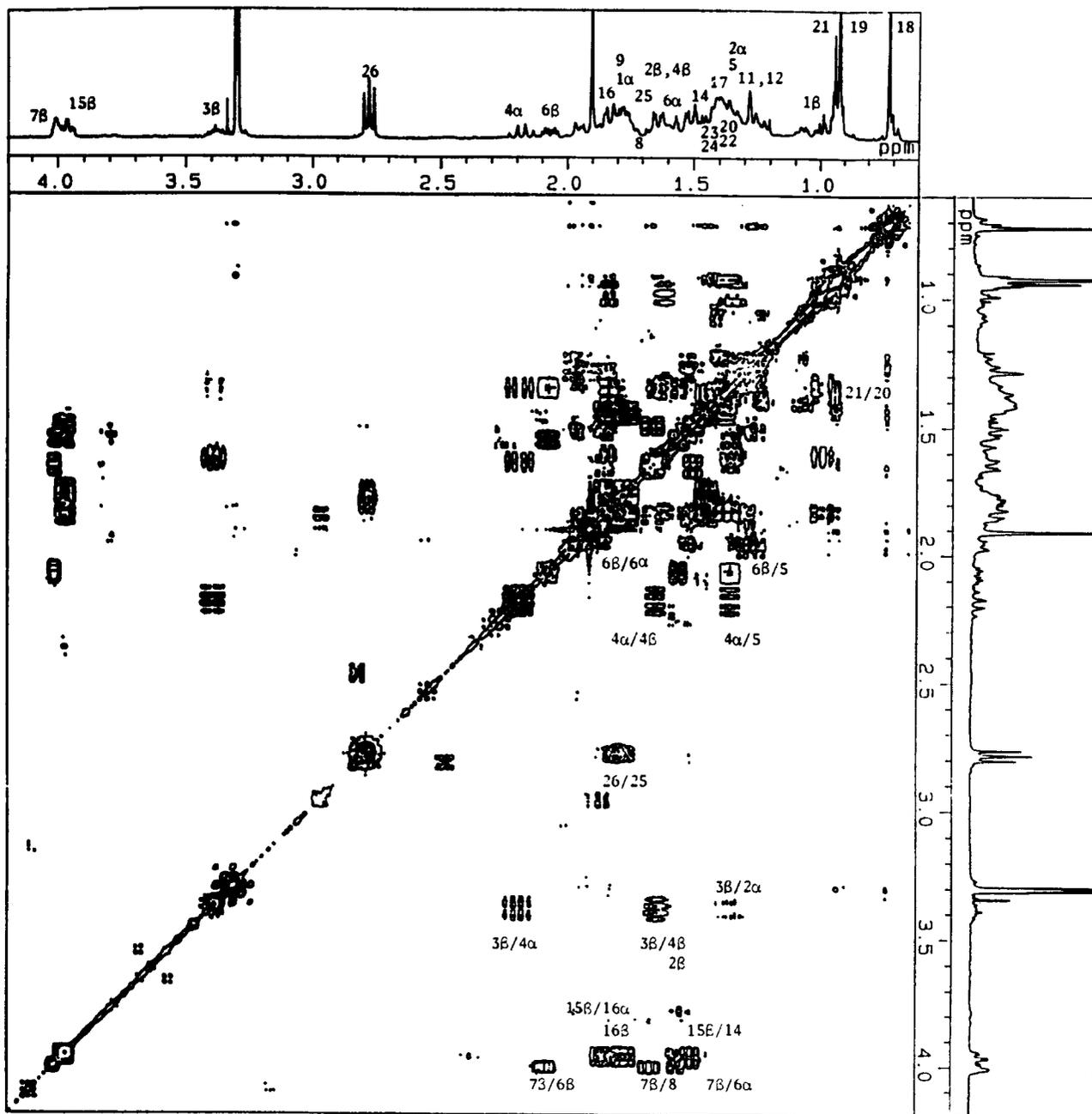
Fig. 4. H,H-COSY spectrum of the major metabolite in  $\text{CD}_3\text{OD}$ . The signal at 1.9 ppm is a solvent impurity (acetic acid or sodium acetate).
